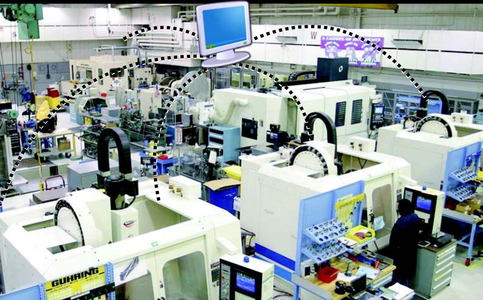
NCnet DNC system transfers programs between a PC and multiple CNC machines through a wired or wireless network.
